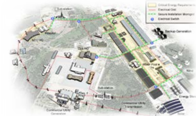
Fort Campbell, KY: MILCON Conceptual drawing a microgrid included in the FY2018 NDAA
